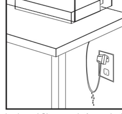
the plug or receptacle does get wet, **DO NOT** unplug the cord. Disconnect the fuse or circuit breaker that supplies power to the appliance. Then unplug and examine for presence of water in receptacle.
